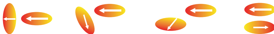
Fig. 1.5 Illustration of the arrangement of the dipole and the induced dipole for various orientations of the two molecules. In each pair, the induced dipole is represented by the smaller of the two arrows. Note that the closest contacts are always between red regions ( \delta^+ ) and yellow regions ( \delta^- ), which means that the interaction between the two dipoles is always favourable.
